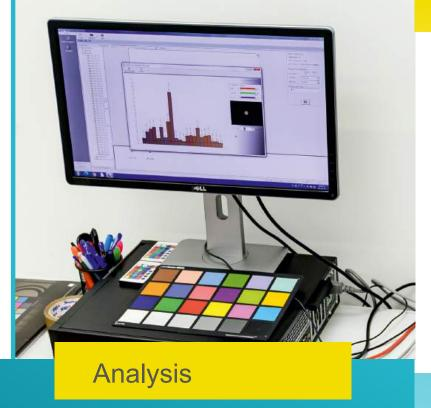
The analysis with IRIS instrument consists of taking a picture using the complementary metal-oxide semiconductor technology camera operating with RGB and L\*, a\* and b\* parameters of the spectrum classification. The pictures are then processed as a color spectrum, with the surface of each significant color calculated in percentage.
