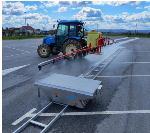
Figure 3 Surface distribution check with spray scanner
