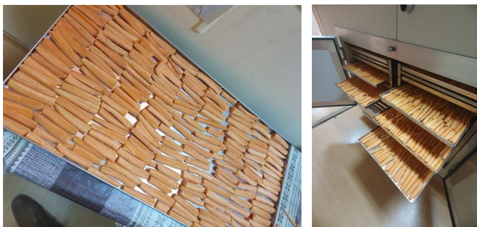
Fig. 2. Fresh carrots disposition on the trays (left) and the shelves arrangement in the condensation dryer (right).
