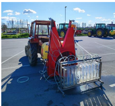
Figure 4 Nozzle flow check for air assisted sprayer
