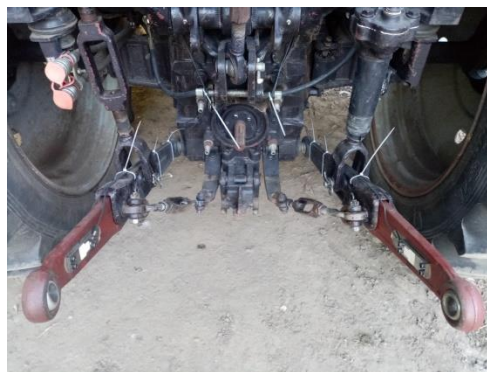
Fig. 2 View of the strain transducers from the inside of the lower levers
