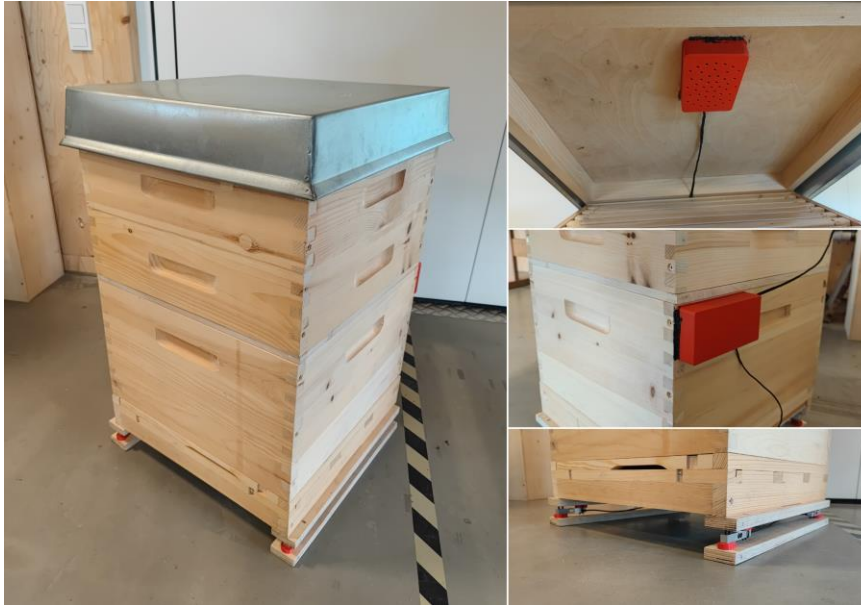
Figure 4. Data acquisition sub-system installed on beehive (left) collecting data of temperature, humidity, sound, vibration (top-right), and weight (bottom-right) with MCU (center right)
