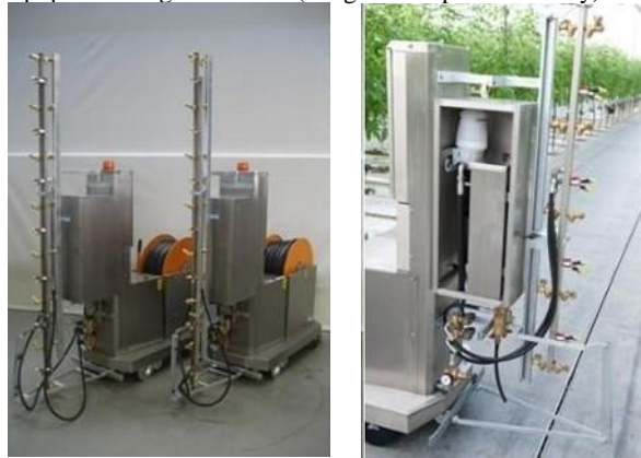
Figure 5 Semi - mobile devices for pesticide application in greenhouses
