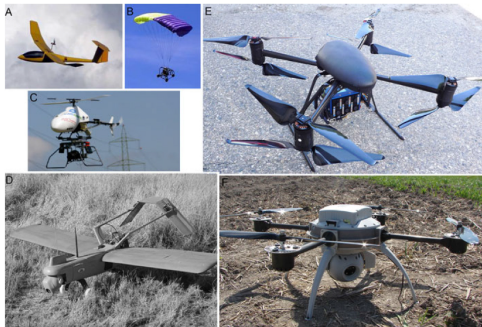
Fig. 1. Various types of USA: A) powered glider, B) powered parachute, C) helicopter, D) fixed wing aircraft, E) dragonflyer X8 quadrocopter, F) aeryon Scout quadrocopter (from Zhang and Kovacs, 2012).
