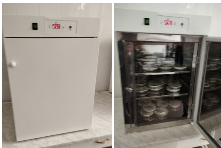
Figure 5. Dry-air thermostat TS-80.
