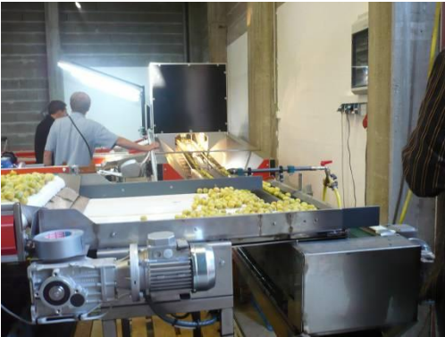
Figure 6. Optical grading line at a private operation near Mainz (1 ton per hour).
